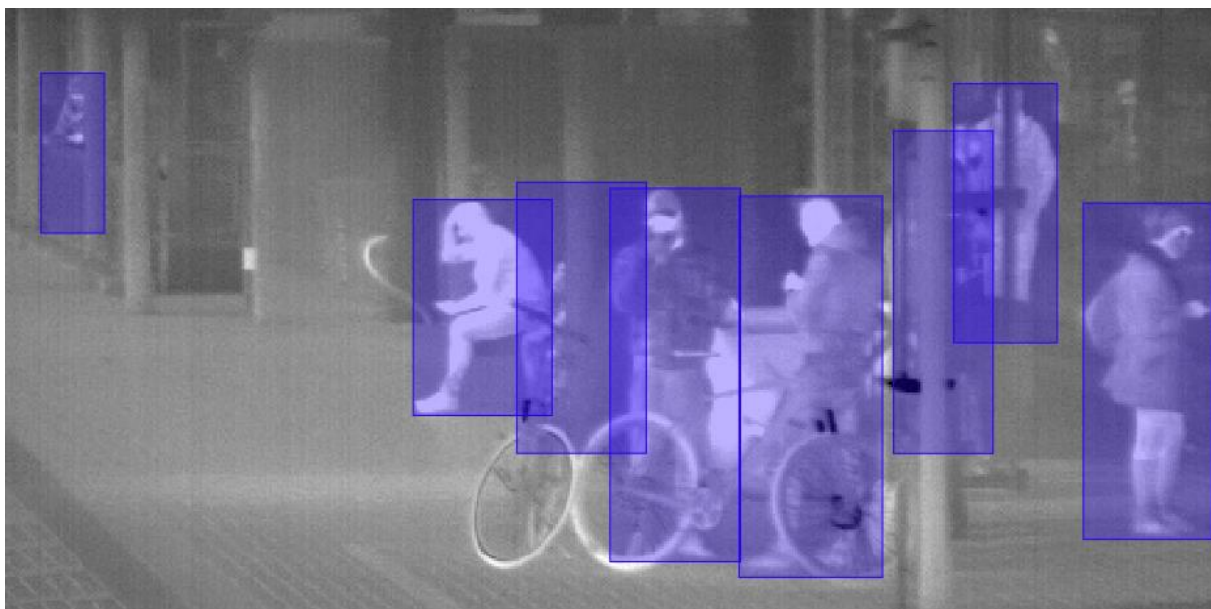
Example for correct annotation of persons in Infrared cameras
