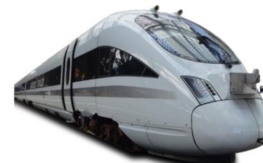
The Advanced TrainLab has a diesel-electric drive system, which enables test rides with a top speed of up to 200 km/h anywhere in DB's railway network. The 107 meter long train consists of 4 wagons, one equipped with the sensors and recording system of the CLUG project.
