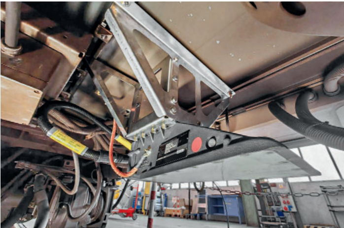
Doppler radar for odometry on one of the first-of-class multiple units (photo: Alstom).
