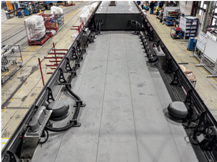
Three elevated antennas on the roof of the Class 430 multiple unit (to the left at the front and rear for FRMCS, to the right for public mobile radio) (photo: Alstom).
