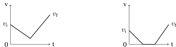
Figure 4: Two possible trajectories for maximal running time: If there exists a trajectory with velocity 0 (right), then the train could wait and the running time is unbounded. Otherwise, the maximum deceleration and acceleration is used as the slowest trajectory (left).
