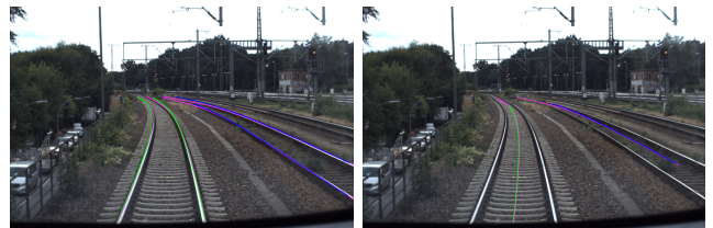
Fig. 1. Rail track detection result with the proposed framework. On the left, the rails, on the right the derived center line. Depicted in green are the outer rail edges of the ego-track, in blue those of the right neighboring rail track and in magenta the ground truth.
